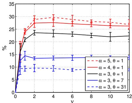
Fig. 8: The fraction of transmitting nodes under the SINR threshold model weighted by the  $x$ -progress.
