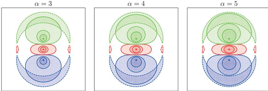
Fig. 1: The areas where a reception is possible for three transmitters (dots) under the Boolean interference model (dashed lines) and the SINR threshold model with threshold 1 (outermost solid lines). The inner solid lines are contours for SINR values 7 and 31.
