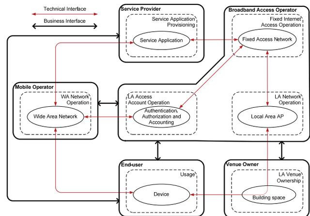
Figure 4. Broadband Access Operator driven VNC.
