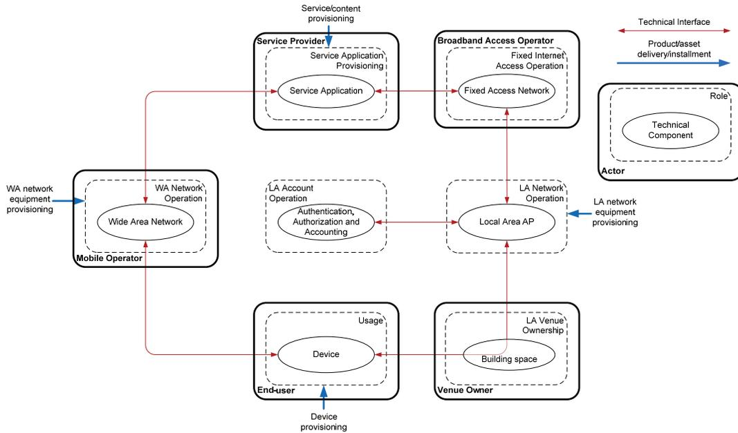
Figure 1. Generic role configuration for wireless local area access provisioning.
