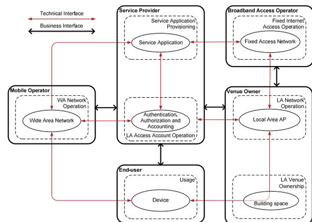
Figure 7. Service Provider driven VNC.
