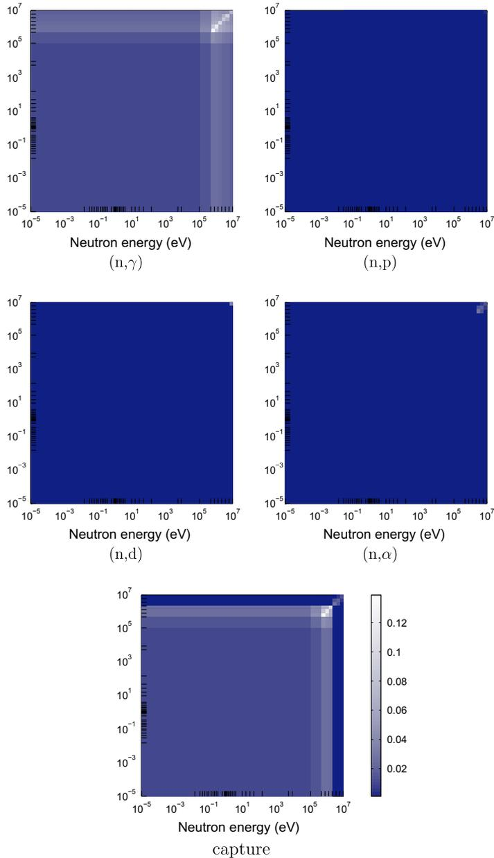
**Fig. 1.** Covariance matrices corresponding to the individual capture cross-sections and the total capture cross-section of  $^{160}\text{O}$ . The covariance matrices in this example are from the SCALE 5.1 covariance library `44groupv6rec` and they have been processed to conform to the energy-group structure of CASMO-4.
