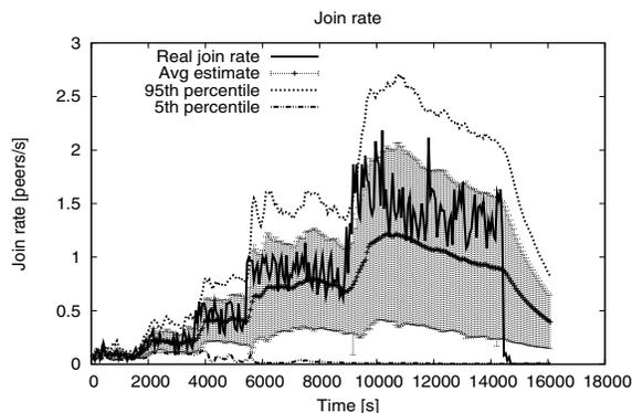
Fig. 2. Join rate estimate, configuration 1 - basic
